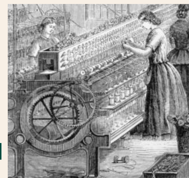
g Doubling-frame which converted yarn into sewing cotton. (Illustrated Times, 1862).
